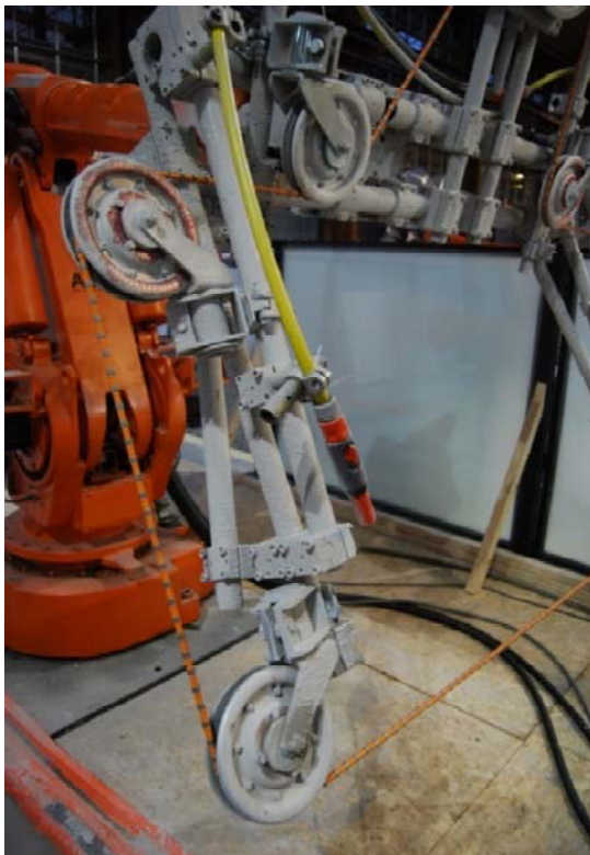
RobArch 12. Left) Abrasive diamond wire cutting end-effector. Right) A section of an asymmetric vault in composite limestone. Source: Author
