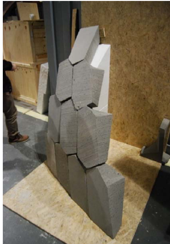
RobArch 12. Left) Abrasive diamond wire cutting end-effector. Right) A section of an asymmetric vault in composite limestone. Source: Author
