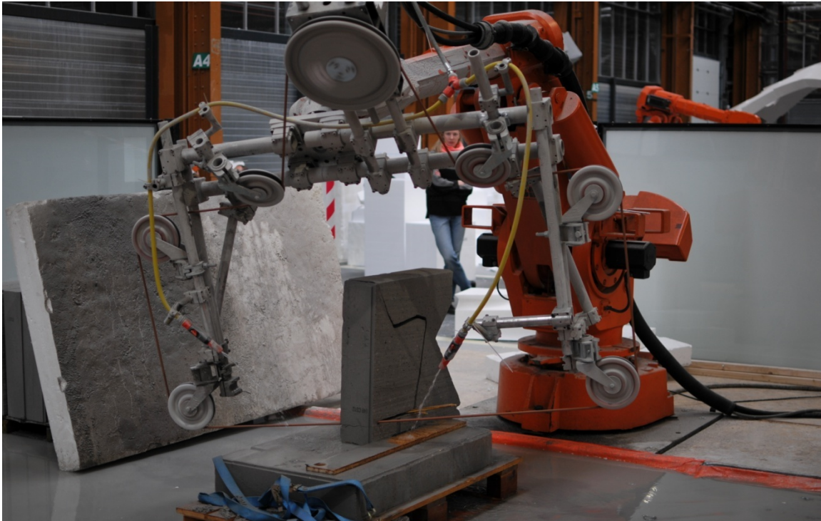
RobArch12: Water outlet still needed to reduce frictional heat and dust particles. Wooden wedges need to be inserted to avoid unwanted splitting. Source: Author
