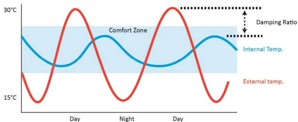
Thermal mass benefits in relation to indoor/outdoor climate. Source: www.greenspec.co.uk
