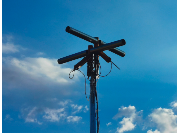
FIGURE 8: The two identical adapted shorted dipoles shifted by 90^\circ in the horizontal plane.
