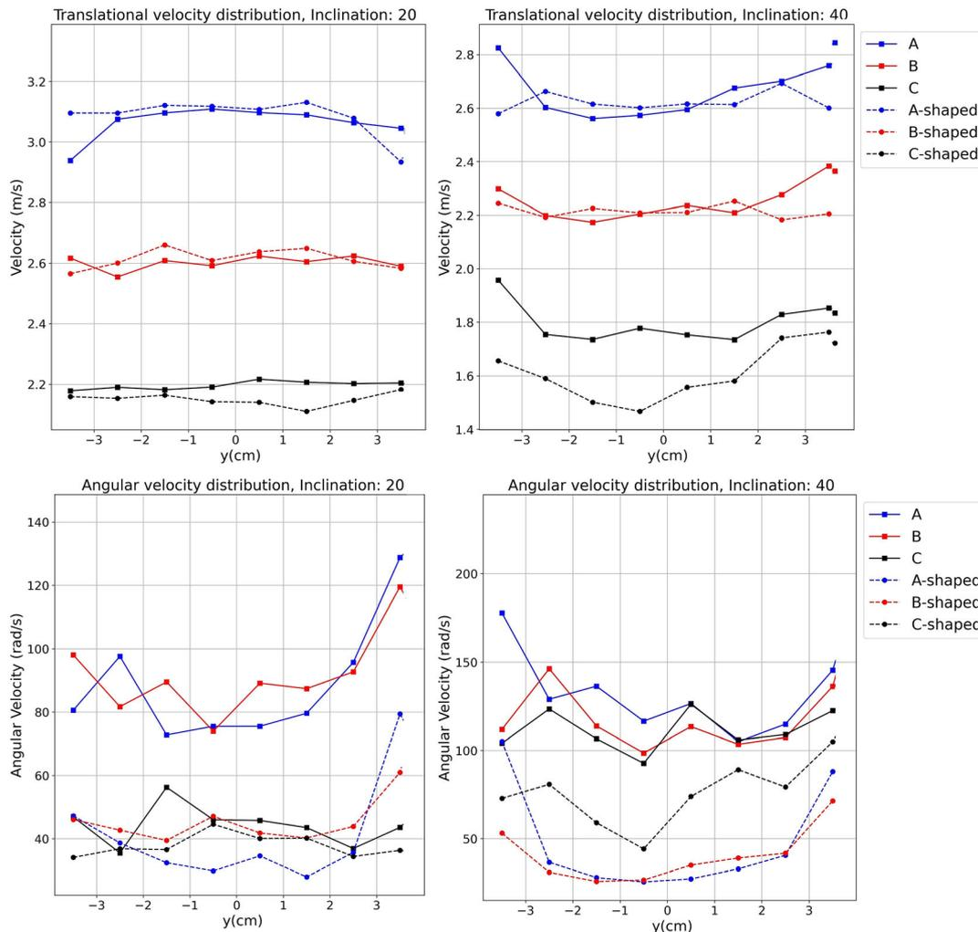
**Figure 15.** Comparison of the translational (top) and angular velocity (bottom) profiles as they have been determined by the spherical and actual shape (shaped) simulation approaches for a batch size of 1 kg.
