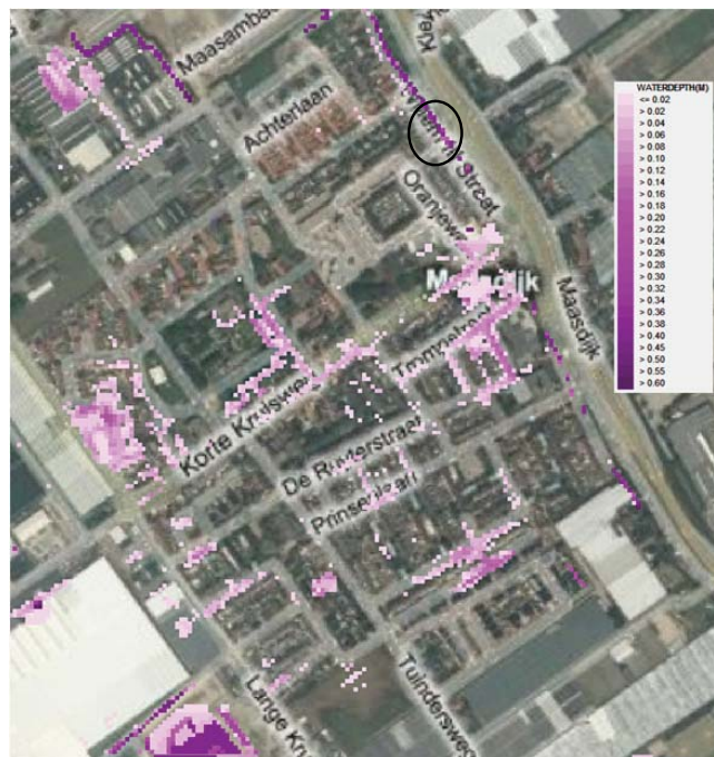
Figure 4.5: Inundation in urbanized area
