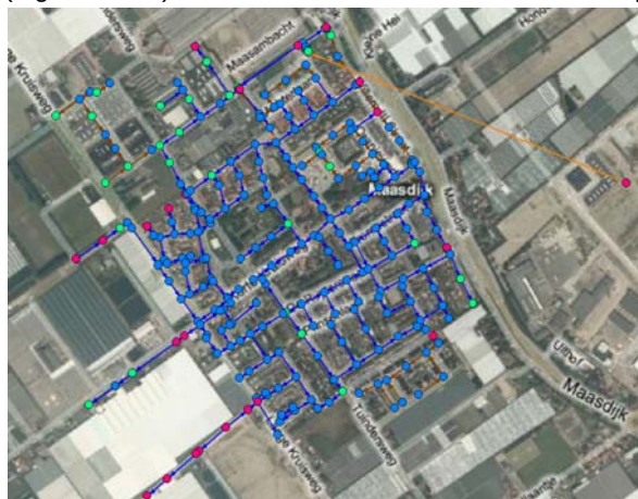
Figure 3.13A: Urban rainfall runoff, sewer flow model
