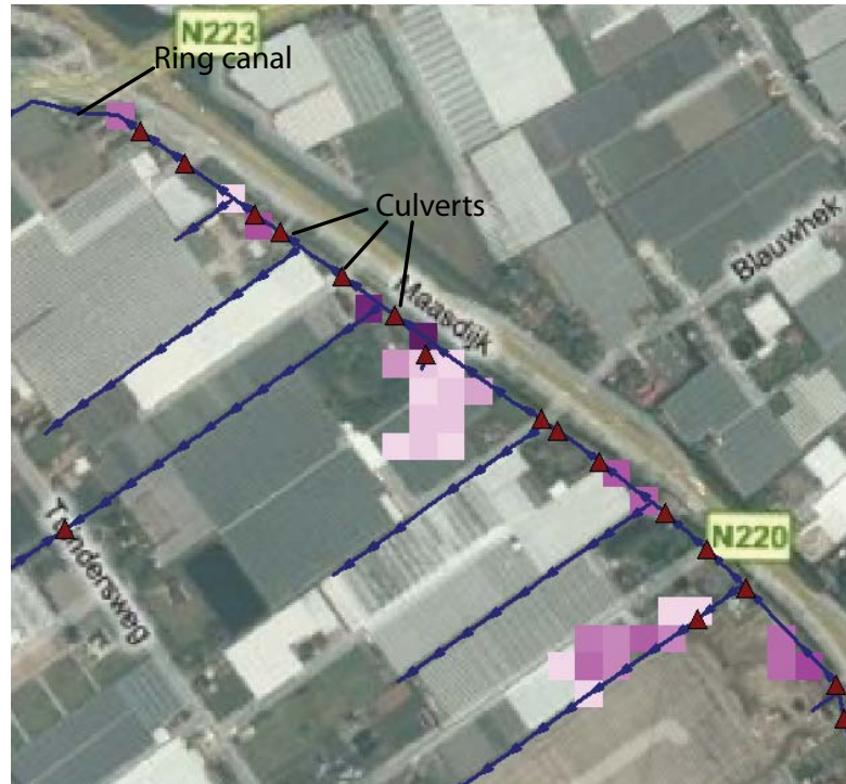
Figure 4.3: Inundation from ring canal caused by head of culverts
