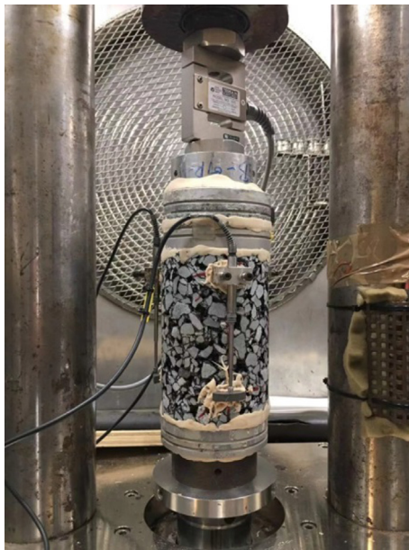
Fig. 9. Uniaxial cyclic compressive tests for PA mixes.
