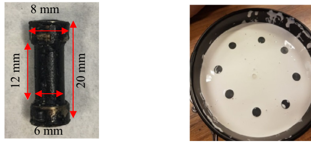
a. Mortar specimens' dimension b. Mould for making mortar specimens
