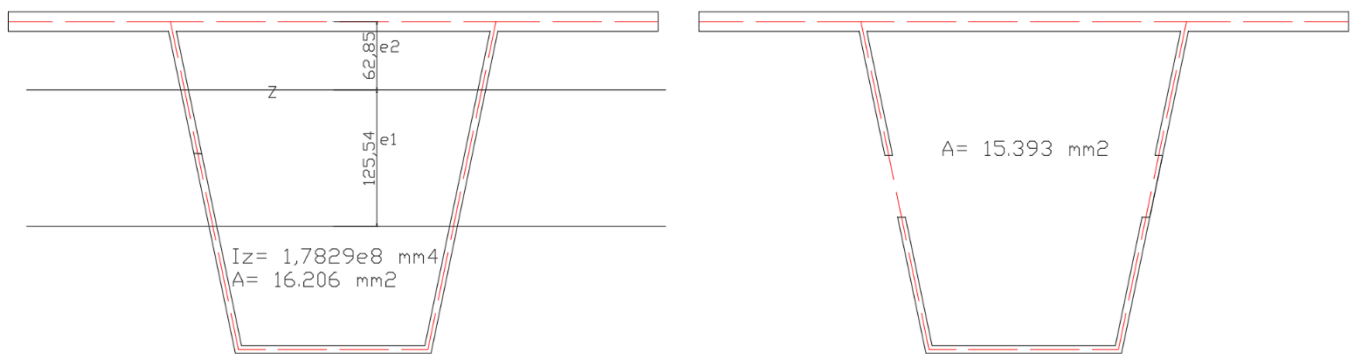
Figures 4.6a, b: Full and reduced relevant inner stiffener properties
