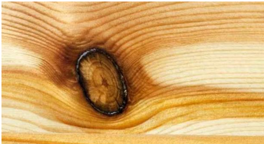
Figure 6.3: Knot in wood, from [ The Pros and Cons of Knots in Wood - Wagner Meters ]
