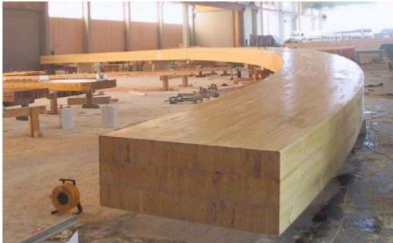
Figure 6.6: Curved Block glued Glulam Member, from [24]
