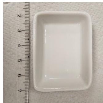
Figure 3.2: Picture of ceramic sample container used in the tube oven.
