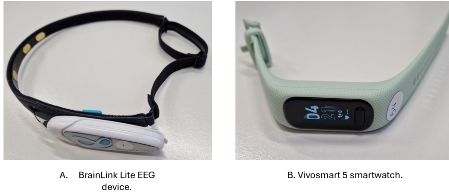
FIG. 5.2 Wearable sensor devices for measuring AL, MRL, HR, and RR.
