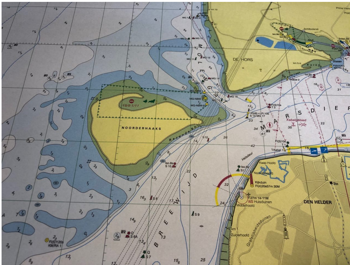
Figure 13.1: An example of an ENC (electronic navigational chart) in the Netherlands. [photo of a paper map from the Hydrografische Dienst ]
