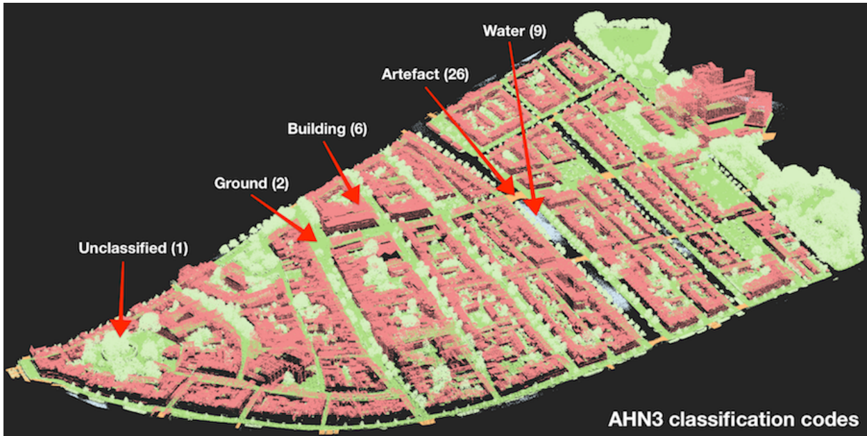
Figure 12.3: Classification codes used in the AHN3 dataset.
