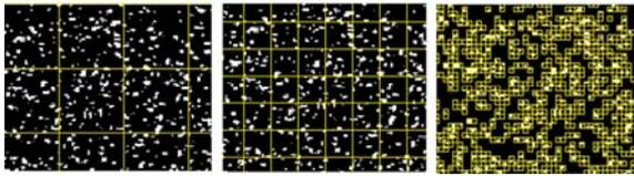
**Fig. 1.** Box counting for a typical speckle image which has been converted to a fractal image. Three different values of box size are shown.
