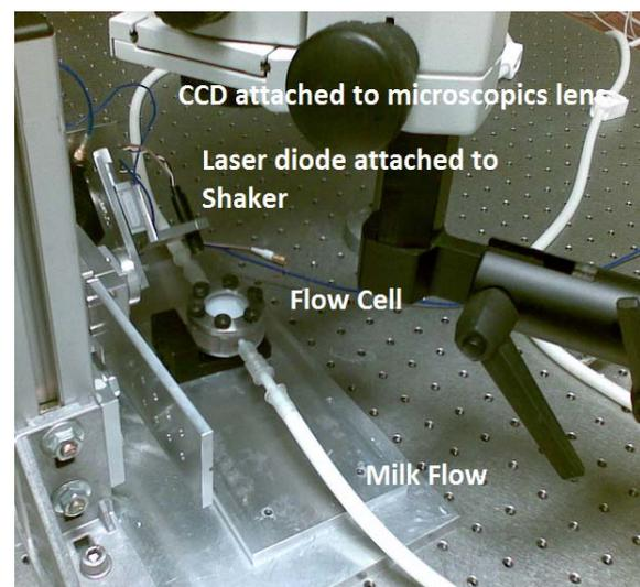
**Fig. 3.** The experimental setup which has been used for the experiments. The flow cell can be fitted with different top membrane to introduce static scatterers. The insert into the flow cell mimics a homogeneous thin layer of flow.
