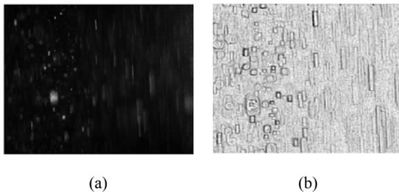
**Fig. 2.** (a) Raw speckle image of pulsatile flow on the left. (b) The speckle image converted to corresponding fractal image, on the right.
