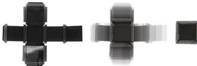
Figure 2.1: An initially flat printed structure is transformed into a three-dimensional closed cube by submerging it into water, causing active material in the hinges to swell (Tibbits, 2014).
