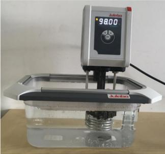
Figure 7.5: Open heating bath circulator
