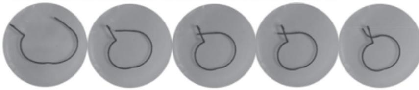
Figure 2.2: Self-locking of a clamp (Inverardi et al., 2020)
