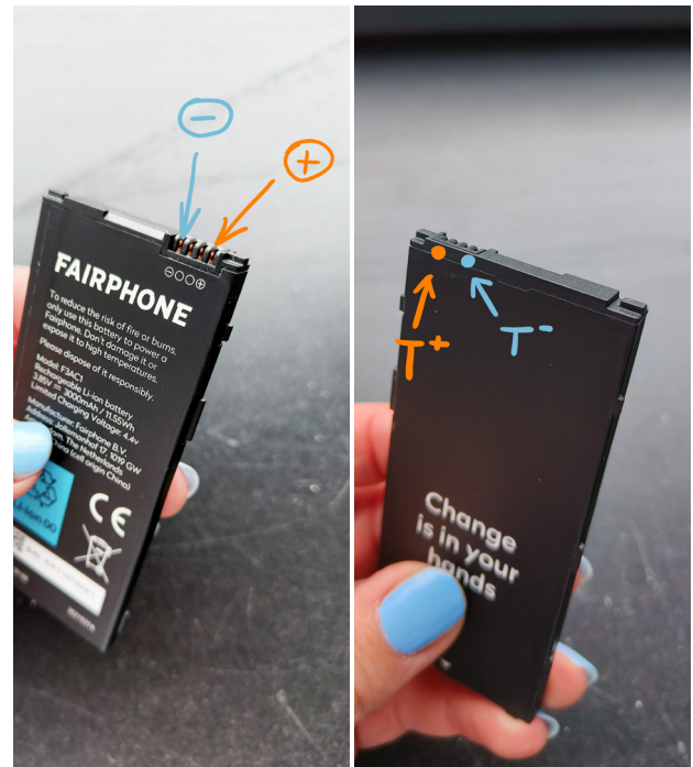
Figure 47. The testing points (T+ and T-) on the battery.
