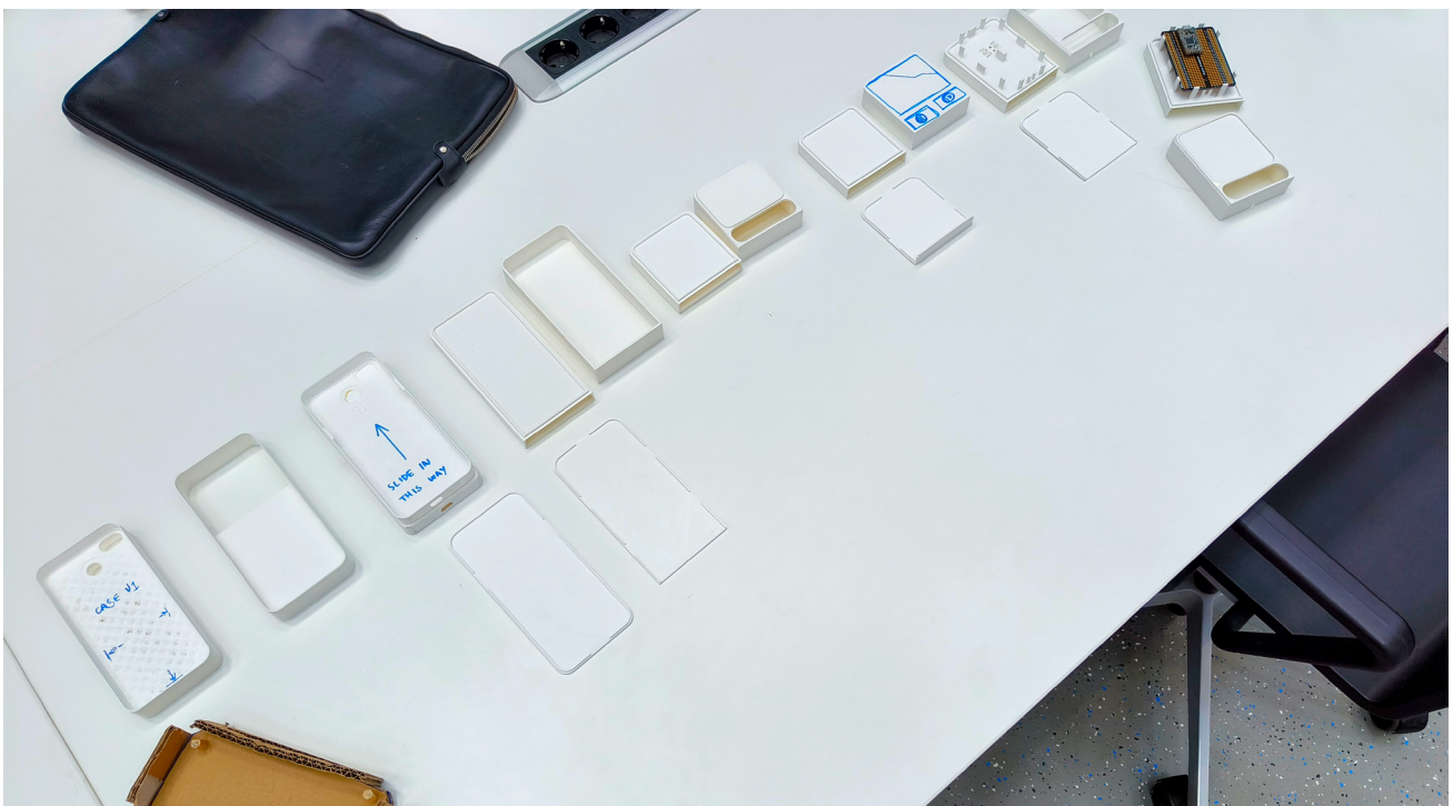
Figure 50. The different form iterations as printed.
