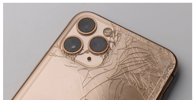
Figure 16. Back cover failure. (Asurion, n.d.)
