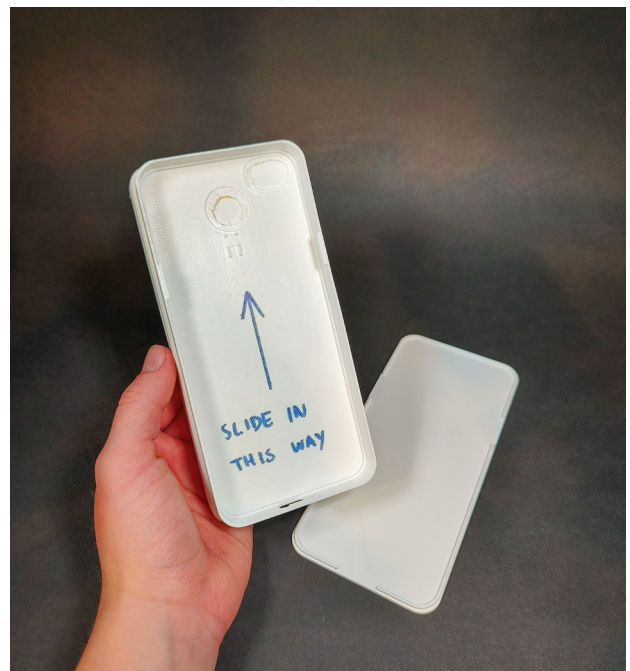
Figure 31. The backside of the prototype where the tested phone slides in.
