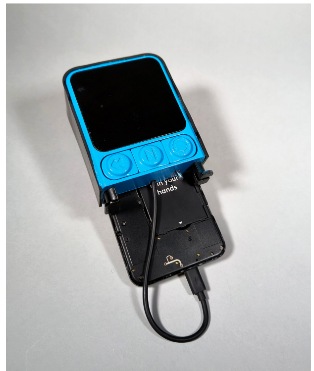
Figure 62. The Fairphone 3 inserted into the prototype.
