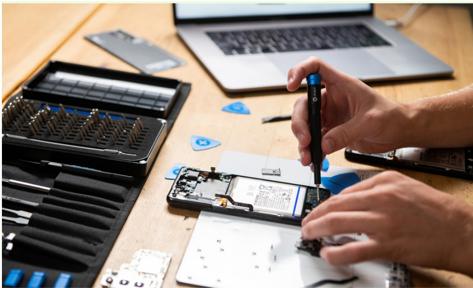
image / figure 1 Repair of a smartphone (iFixit)
