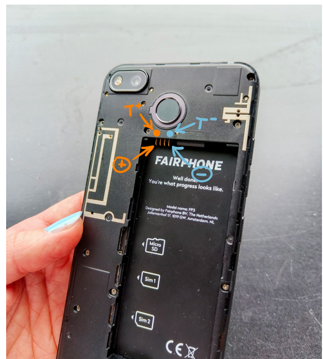
Figure 48. The testing points (T+ and T-) on the battery terminal.
