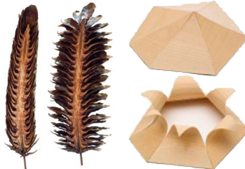
Figure 4 Left: Conifer cones in open and closed states. Right: a responsive system component was developed that can adapt its shape by being based on a four-, five-, six- or seven-sided polygon (Menges and Reichert, 2012). Iva Kremsa, Kenzo Nakakoji and Etien Santiago, Performative Wood Studio (Achim Menges), Harvard University Graduate School of Design (GSD), Cambridge, Massachusetts, 2009.
