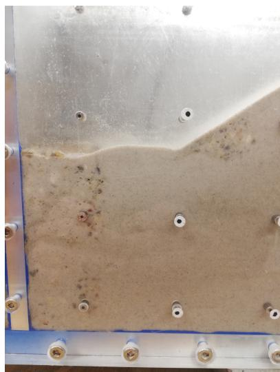
Figure 5.14: filter layer filled with geba sand
