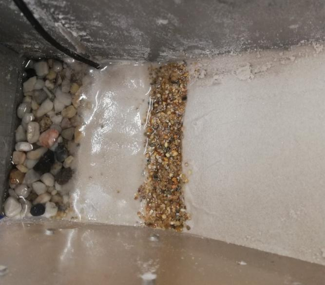
Figure 5.11: topview left side strongbox after remodelling toe and increasing water level
