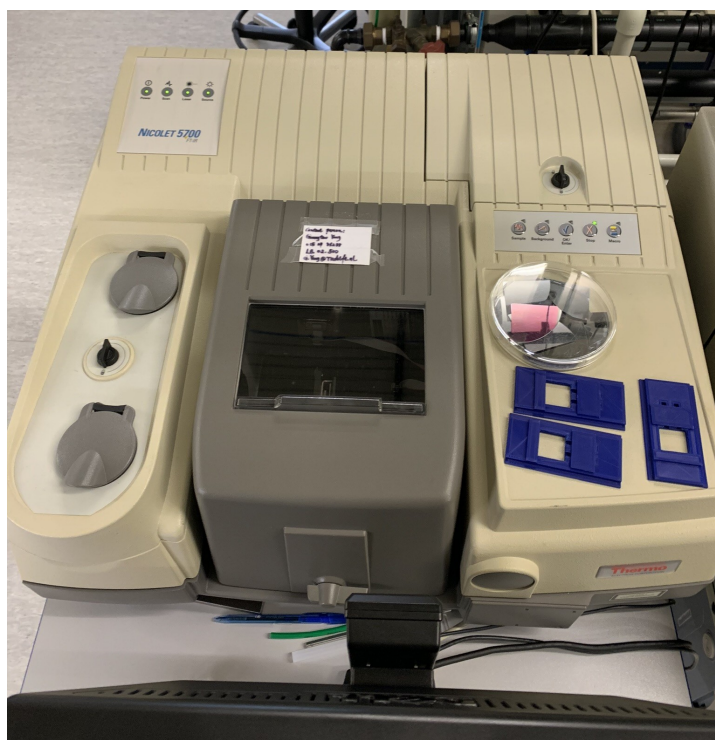
Figure C.6: Picture of the Thermo Fischer Nicolet Fourier Transform Infrared Spectroscopy (FTIR), located in the Else Kooi Laboratory. In the center of the image, the window used to load the sample is visible. The machine has two slots: one for the sample, and the other for the reference substrate or left empty. After opening the window, it is recommended to purge the chamber with nitrogen for at least 15 minutes before starting a measurement. This step helps remove water vapor and ensures a stable background signal.
