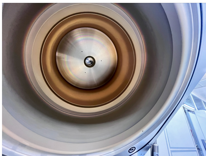
Figure C.3: Top view of the Oxford Instruments PlasmaPro 100 ICPCVD chamber during maintenance. The gas inlet, used for introducing argon in this application, is clearly visible. The ICP coil, responsible for ionizing the gases to generate plasma, is located behind the chamber wall and not visible in this image.
