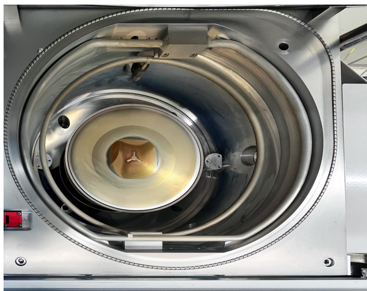
Figure C.2: Chamber of the Oxford Instruments PlasmaPro 100 ICPCVD system during maintenance, with the top section lifted (see Figure C.3) to reveal the bottom half. At the center, the wafer lift is visible, which supports the wafer during processing. Two gas inlet rings are mounted along the chamber wall, through one of which argon and \text{SiH}_4 are introduced into the chamber.
