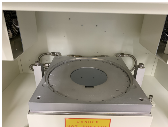
Figure C.4: Picture of the inside of the FLX-2320-S stressmeter system, located in the Else Kooi Laboratory. The wafer is placed at the center of the platform, resting on three pins to minimize contact. The orientation of the measurement is determined by the alignment ring surrounding the wafer. A laser scans along a straight line through the center of the wafer to measure its bow. By comparing the wafer bow before and after deposition, and using the film thickness, the residual stress is calculated.
