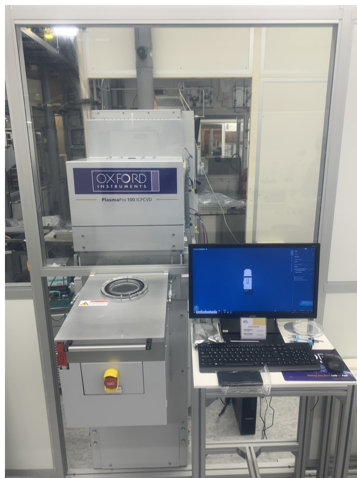
Figure C.1: Picture of the Oxford Instruments PlasmaPro 100 ICPCVD, the ICP-CVD tool used for the thin film depositions. This tool is located in the Else Kooi Laboratory. Next to the computer, which runs the operation software, is the loadlock. When a wafer is loaded into this loadlock, the pressure is pumped down to closely match the high vacuum of the deposition chamber before it is transferred inside. It includes two gas rings, as can be seen in Figure C.2.
