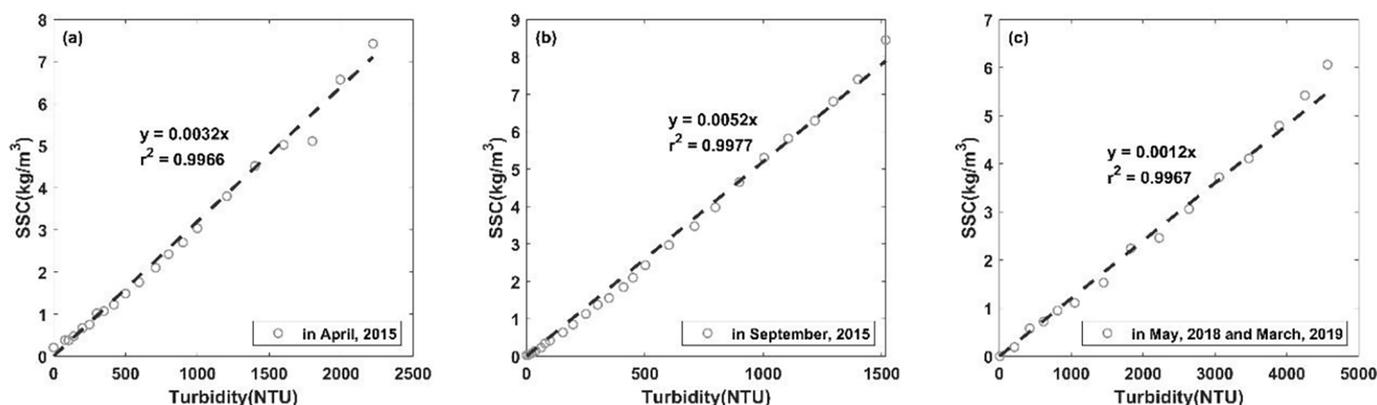
**Fig. A.1.** Sediment calibration curves of the optical backscatter signal with SSC data in (a) the main creek in April 2015, (b) the main creek in September 2015, and (c) the secondary creek in May 2018 and March 2019.
