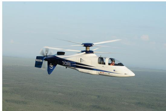
Figure 1.2: Sikorsky X2 demonstrator [5]
