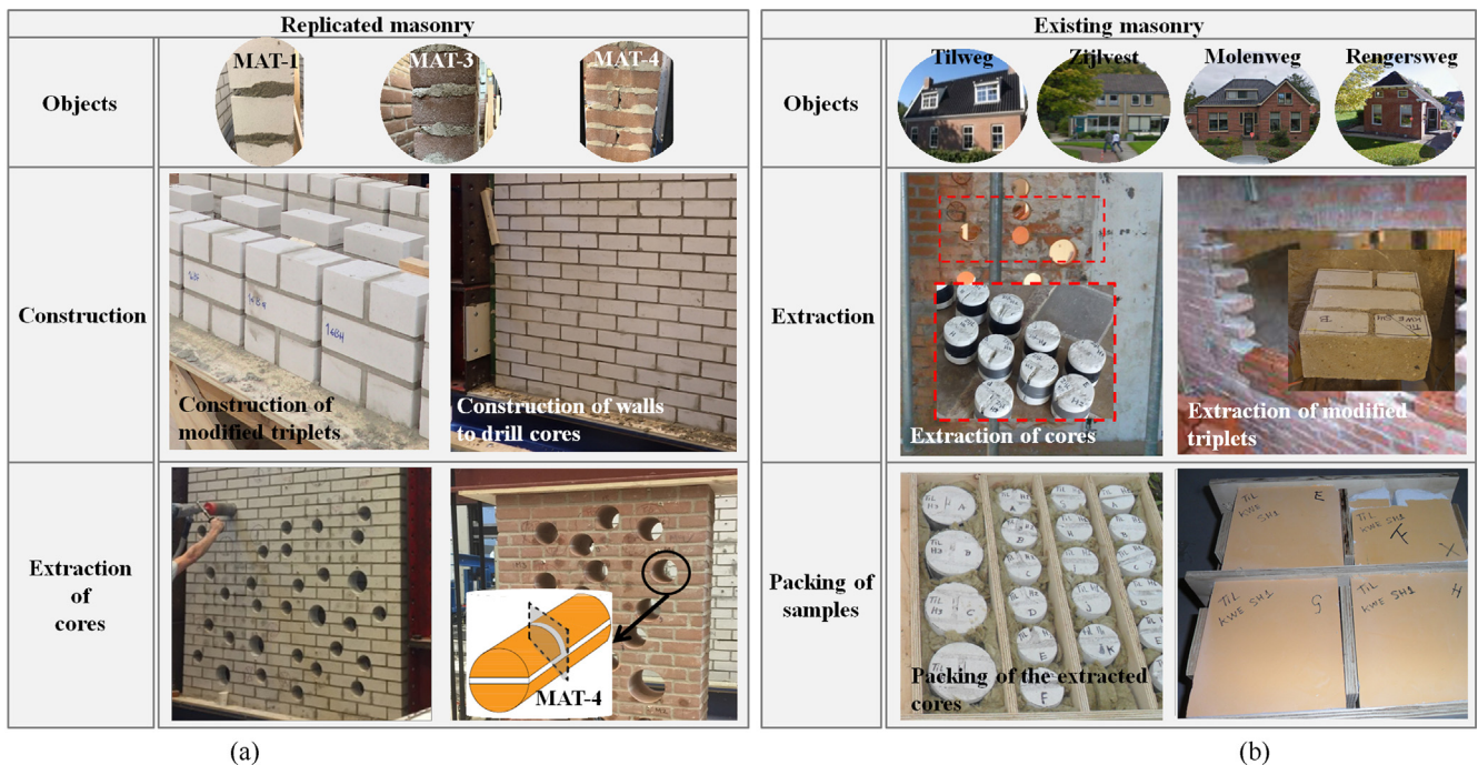
Fig. 2. Overview of the masonry objects: (a) replicated in laboratory; (b) extracted from existing buildings.
