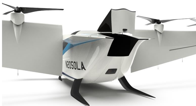
Figure 8.1: The Bumblebee EX has a rear loading trunk that fits two full-size suitcases. Below the trunk is the charging port.
