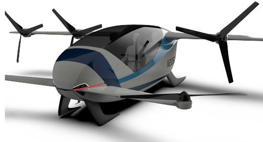
Figure 8.7: Red lights on the fuselage indicate the vehicle is not safe to approach. The lights turn green when it is safe to approach.
