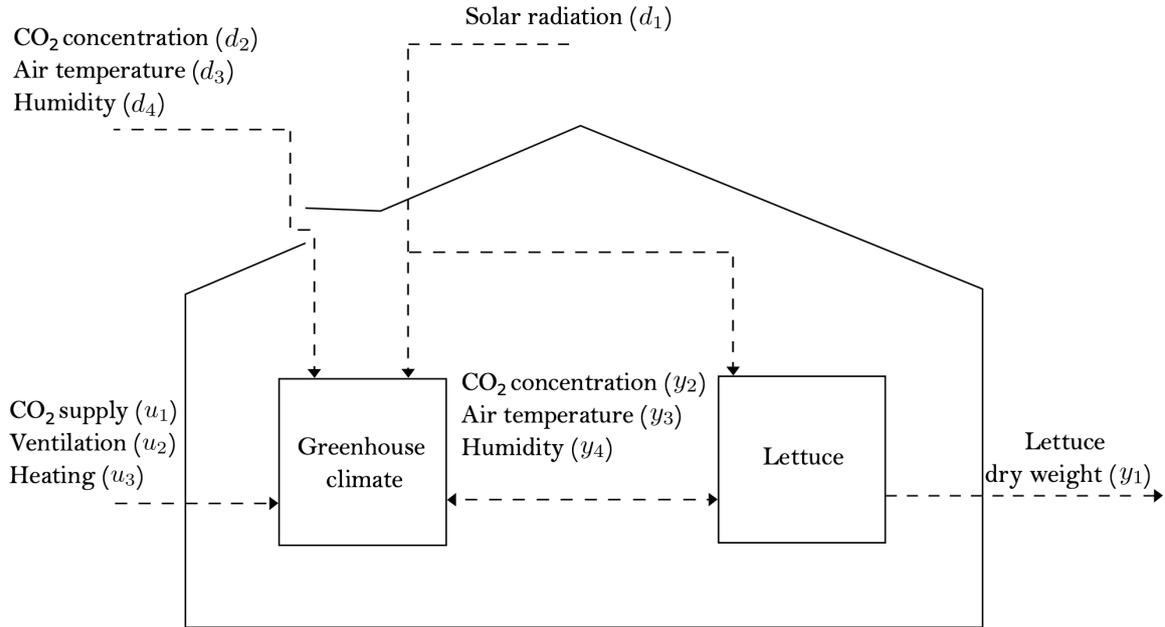
**Figure 3-1:** Greenhouse with lettuce schematically represented. The interaction between the greenhouse and lettuce model is indicated with the arrows. The influence of the control signal  $u(k)$  and weather disturbance  $d(k)$  are also indicated by the arrows. The figure is taken from [48].
