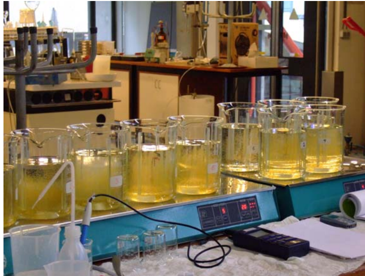
Figure 5.2 – Mixing beakers with resin inside (batch experiment)
