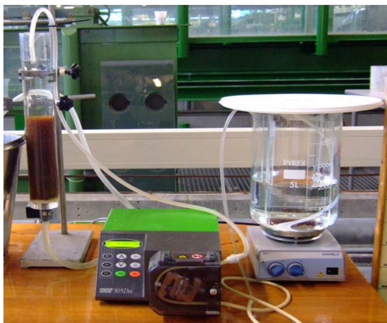
Figure 5.5– setup for regeneration and production
