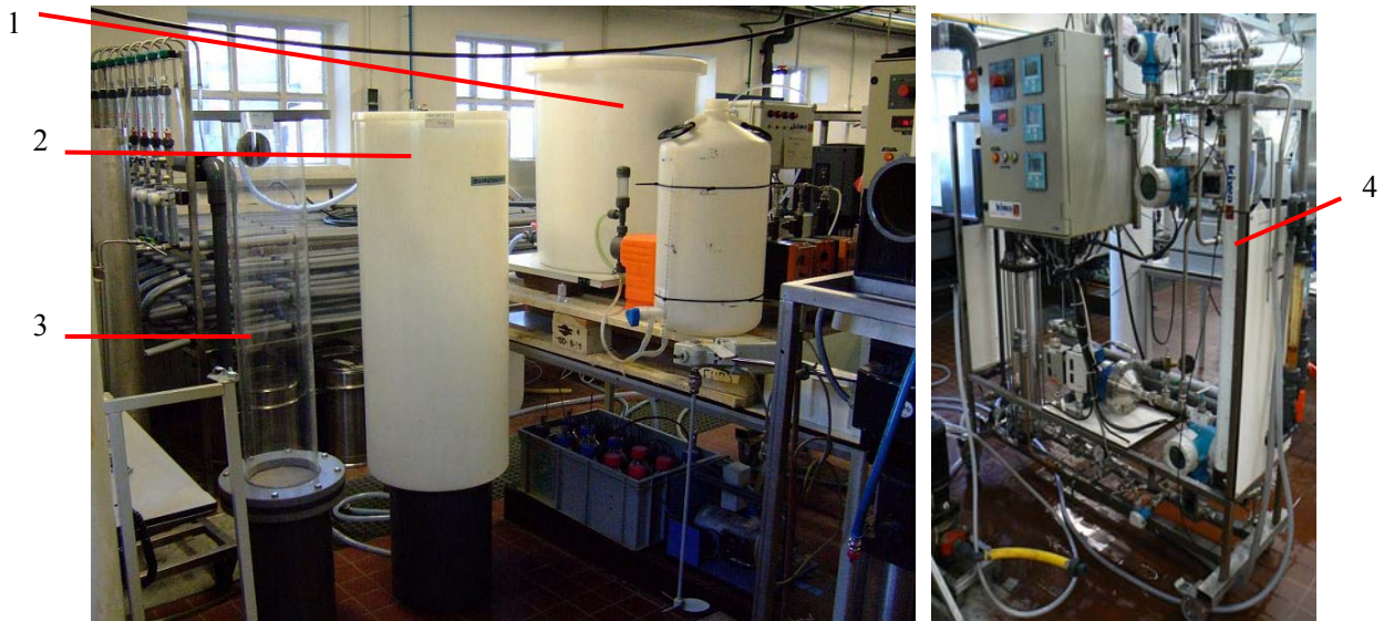
Figure 3.2 – Picture of the equipments 1) Sludge softening vessel; 2) Sedimentation tank; 3) Ion exchange column 4) Nanofiltration membrane module
