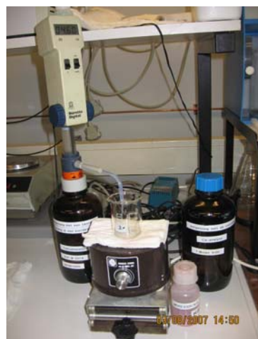
Figure 5.3 – Setup for calcium analysis
