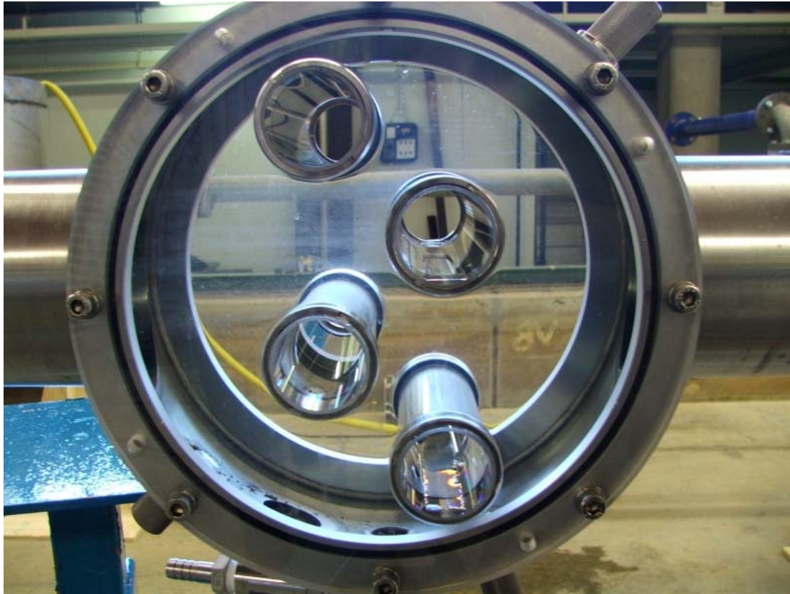
Figure 6-1 Picture of the UV reactor with transparent flanges (inflow water direction: left to right)
