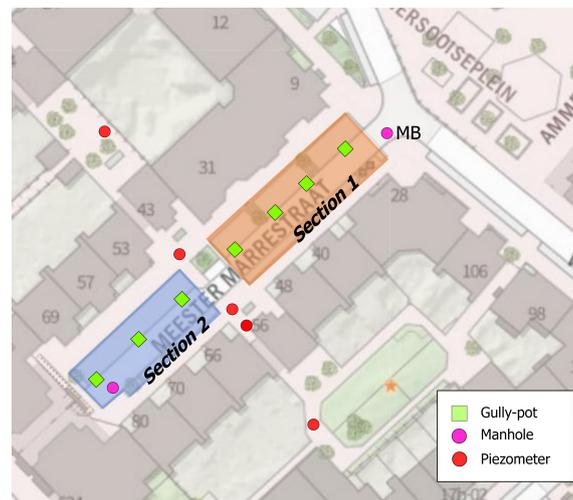
**Figure 5.3:** Sections for full scale test load discharge
