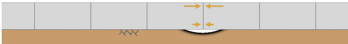
Figure 5.13: Settlement of the soil without deformation of the tunnel segments
