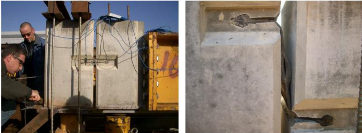
Figure 6.16 - Testing the rubber profile of an segment joint [67]
