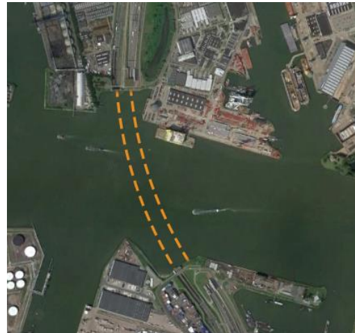
Figure 2.14: The horizontal alignment of the Beneluxtunnel [5]
