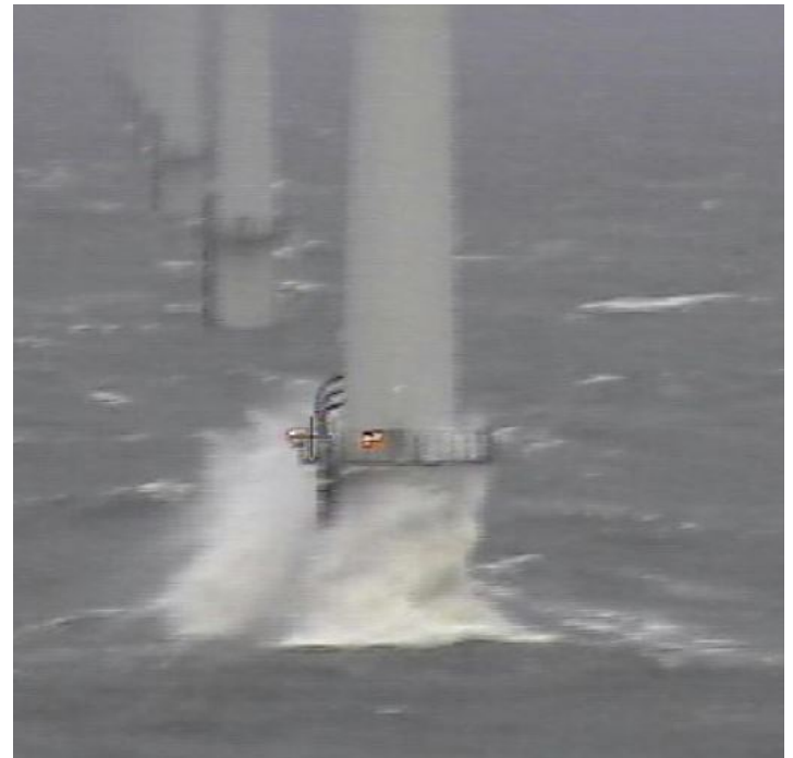
Figure 1: Wave run-up at Horns Reef (Damsgaard, Gravesen, and Andersen, 2007)
