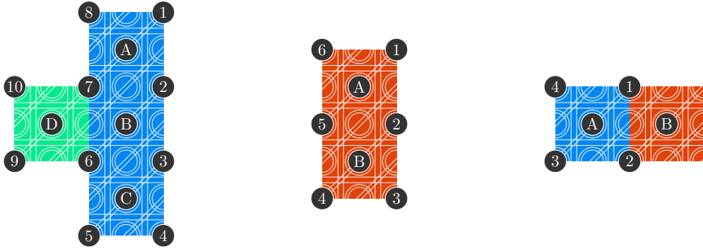
FIG. 12. Unit cells of the deformed 4.8.8. and 6.6.6. codes (left and middle respectively) and the unit cell of the surface code ( Z -cycle) with the gray circle corresponding to qubits. For the 4.8.8. unit cell the qubit labeled ‘A’ is the ancilla qubit for the octagon (now a rectangle) sub-cell while the qubit labeled ‘D’ is the ancilla for the square sub-cell. The qubit labeled ‘B’ is used to read out the qubit labeled ‘D’ and the qubit labeled ‘C’ is used to read out the ancilla qubit for the octagon cell directly below the square cell (not pictured). The qubits labeled by numbers are the data qubits. For the 6.6.6. unit cell the qubit labeled ‘A’ is the ancilla qubit used to perform the stabilizer measurement while the qubit labeled ‘B’ is used to read out the ‘A’ qubit for the unit cell directly to the bottom left (not pictured). The numbered qubits are again data qubits. For the surface code unit cell the qubit labeled ‘A’ is the ancilla used for the Z -cycle stabilizer measurement while the qubit labeled ‘B’ is the qubit used to read out the ‘A’ qubit. It is also the qubit used as the ancilla for the X -stabilizer cycle. The numbered qubits are again data qubits. Note that this unit cell mirrors when moving upwards. That is, the unit cell above the one pictured will have the ancilla qubit B to the right of qubit A instead of to the left as pictured.
