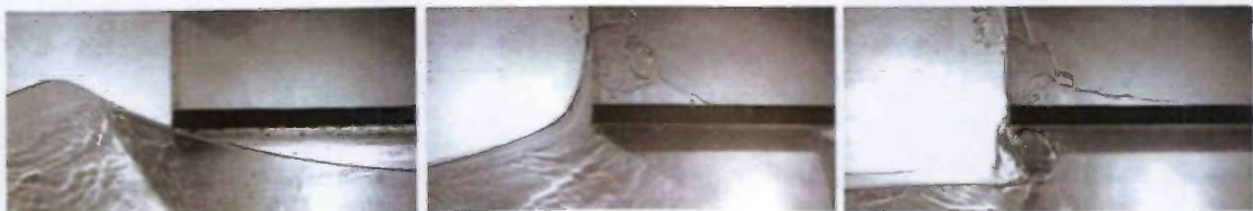
Fig. H11: Snapshots from wave impact experiment. Photo: Rolf Baarholm/Trygve Kristiansen.
