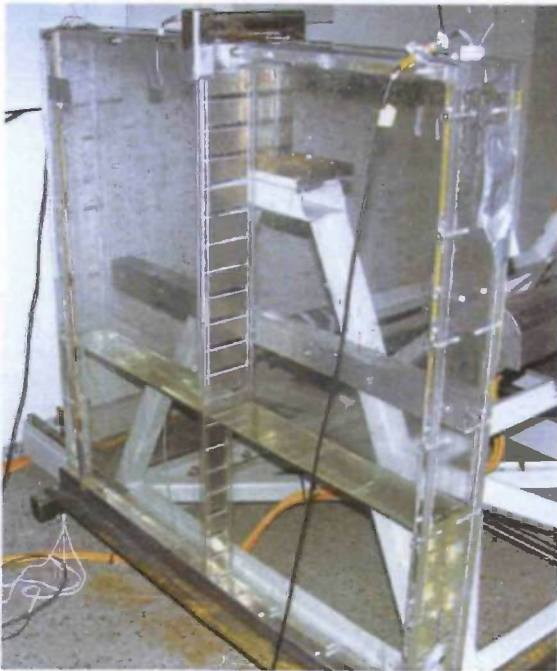
Fig. H5: The two-dimensional sloshing experiments were conducted in a tank with a perforated wall in the centre.
