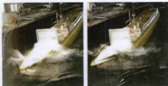
Fig. H2: Water-on-deck experiments: high-speed jet rising at the bow (left) and initial wave-plunging phase during water shipping (right).
