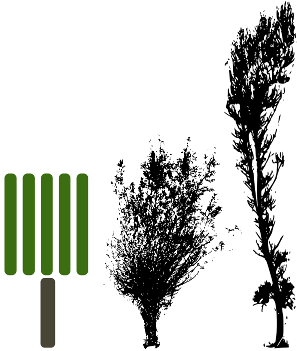
Figure 2: Conceptual comparison between overly simplified vegetation representations commonly used in wave attenuation modelling, and TLS-derived vegetation structure.
