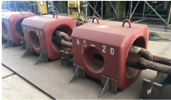
Figure 5.21: Clump weights of a mono-cast design fitted on chain [26]
