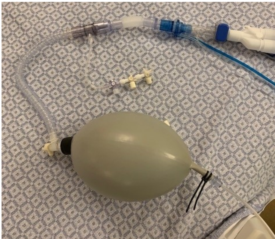
Figure C.2: Close-up picture of the connection from the cylinder to the test lung and from the test lung to the mechanical ventilator and the Masimo.
