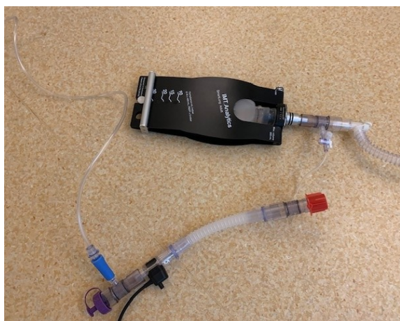
(a) Connection of the IMT Analytics Smartlung Adult test lung to the cylinder inlet which was connected with a Sensirion flow sensor to the circuit.
