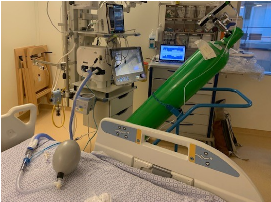
Figure C.1: Picture of the result of the first designed test setup. The green cylinder is connected to the two liter AMBU test lung which is connected to the Hamilton C6 Mechanical Ventilator and the Masimo ISA OR + .
