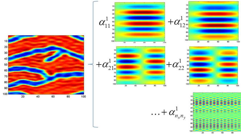
Figure 4 Parameter field expansion with HOSVD
