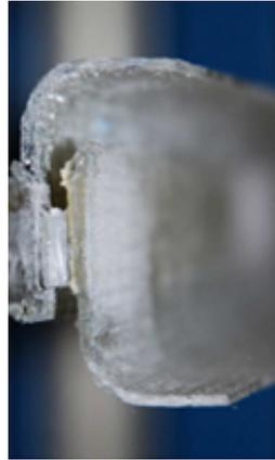
Figure 2.18: Adaptive interface in the front spar of the experimental wing. Adapted from *Raither et al.* [7].
