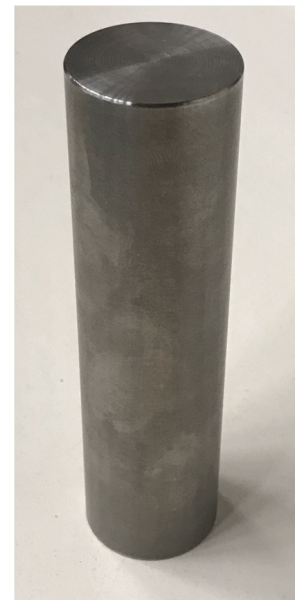
Fig. 13. Aluminium cylindrical objects, ( L_{co} = 100, 120, 160 mm • D_{co} = 20, 30, 40 mm), \rho_p = 2,701 kg/m 3 .
