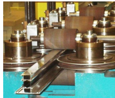
Figure 43 (left) Basic section of aluminium window frame possesses a high structural integrity (right) Assembly of aluminium-plastics composite profile is carried out in shop
