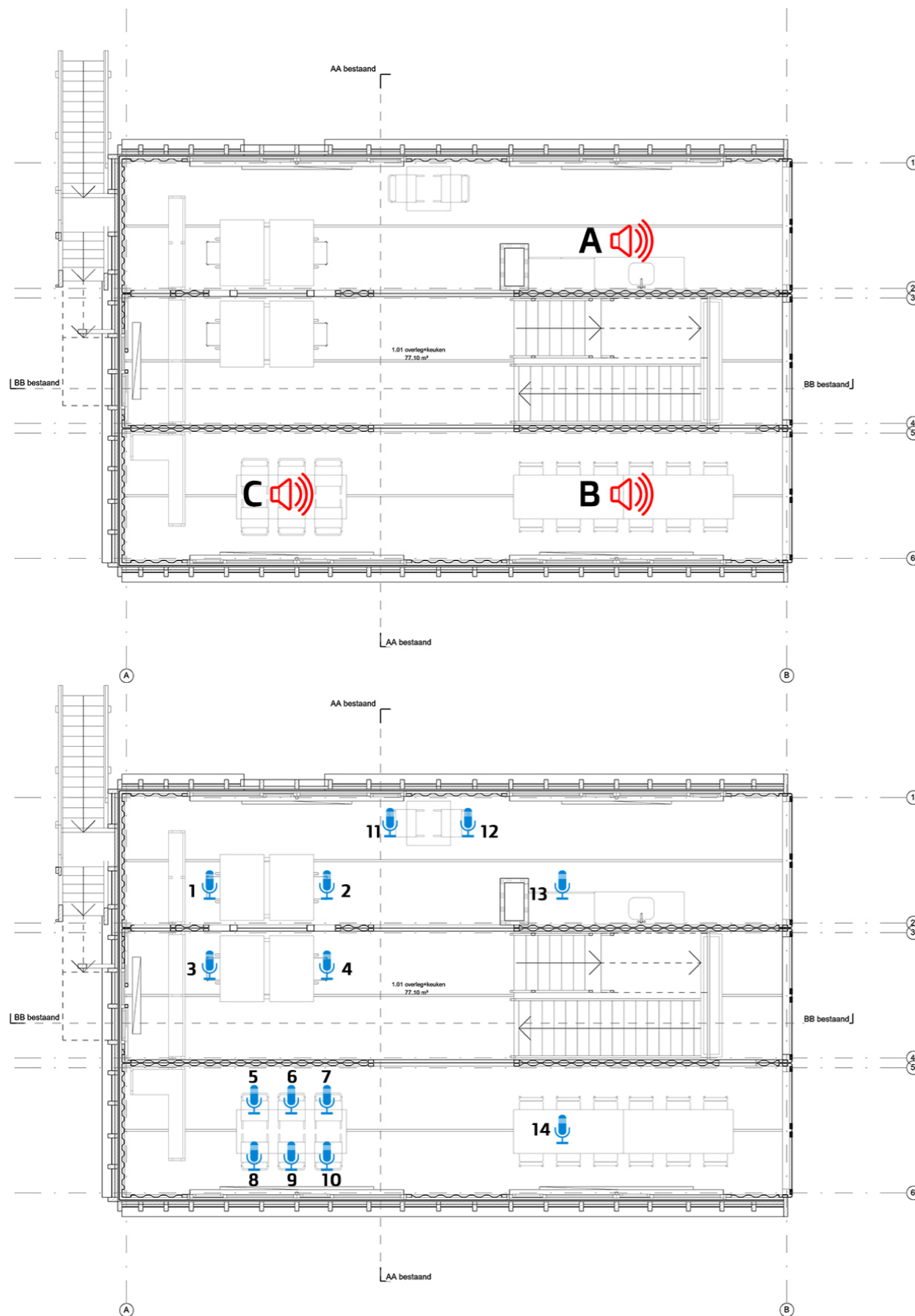
Figure 6.13. Location of source position (top) and receiver position (bottom).
