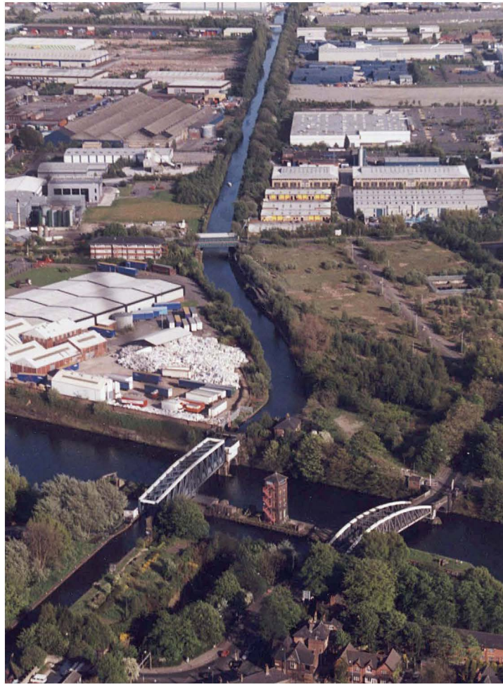
The swing-aqueduct carrying the Bridgewater Canal over the Manchester Ship near Manchester, England.
