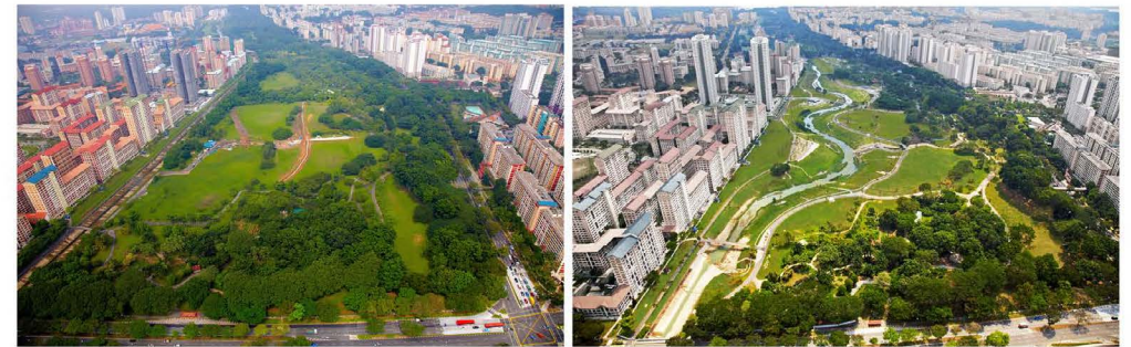
The old Kallang River is an artificial channel to collect and drain the rainwater from nearby urban surface. After naturalized, it has the functions of rainwater purification, ecology and recreation. Photo via wikipedia.
