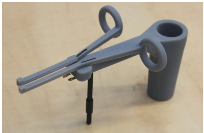
Figure 11. Rapid Prototype models. Top: First set of Rapid Prototype components; two handles and three pair of rods. Bottom: An assembled Rapid Prototype model. The black rod is for support and is not part of the model.
