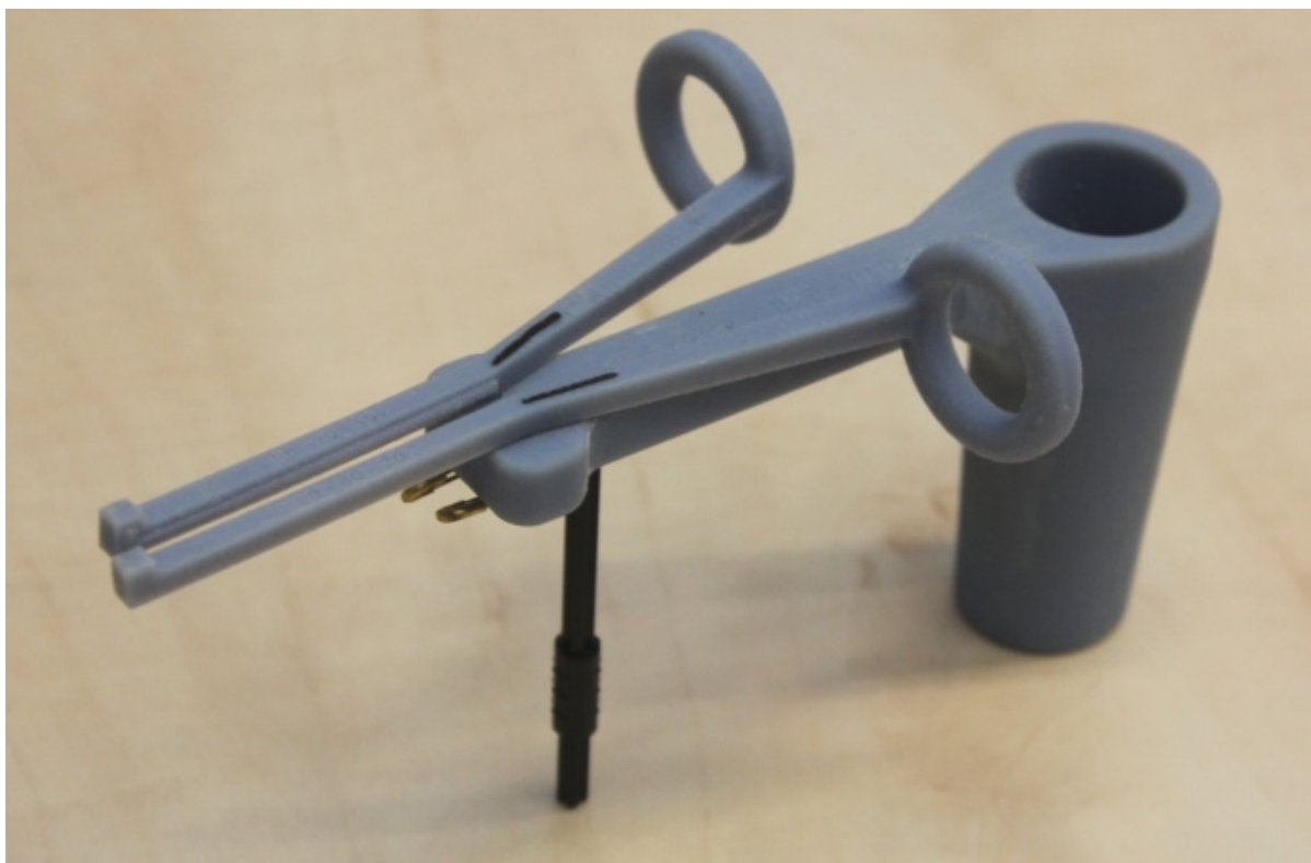
Figure 23. A rapid prototype model with rods from the first set. At the inside of the rods the size of the real rods are printed (difficult to see). The black rod was used as support and is not part of the model.
