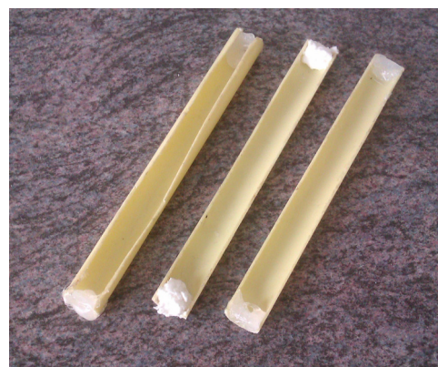
Figure 31. Molds to make a gelatine nerve.
