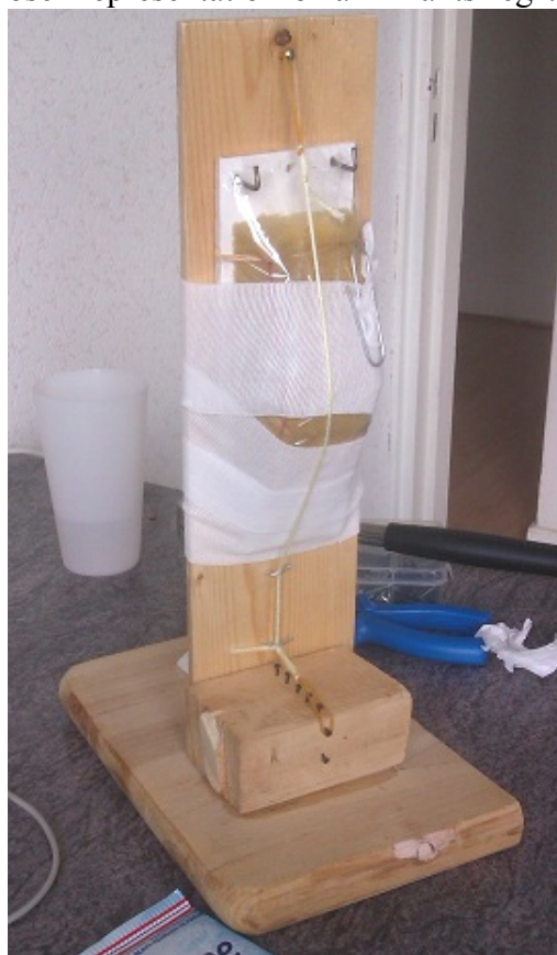
Figure 30. Second test facility. For visual purpose the limited bandage (artificial skin) is wrapped behind the thread (artificial nerve).
