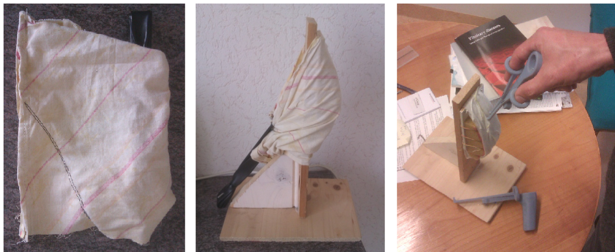
Figure 29. Left: Artificial skin, note the black sewing seam at the bottom left corner. Middle: With the sewing seam and a inner tube the skin is wrapped equally around the soft tissue plate. Right: The surgeon is testing rapid prototype models, he uses the first test facility to give a better feeling and visualisation. The test facility aids him in his decision making.
