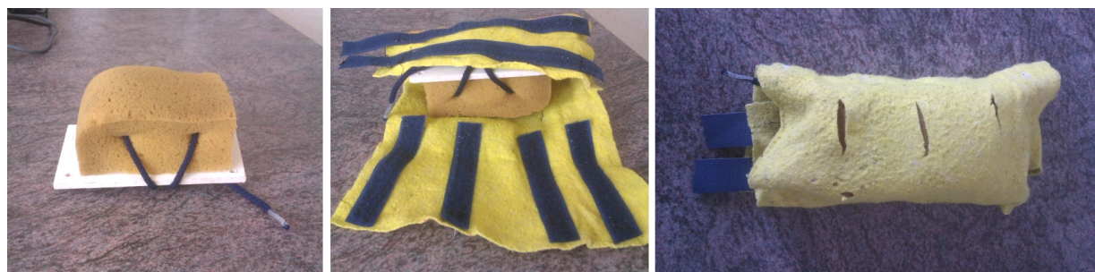
Figure 28. First concept for the soft tissue. Left: plastic plate with sponge. Middle: Sponge wrapped in yellow dishcloth with Velcro. Right: The end result with three incisions.
