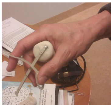
Figure 18. Testing with a salt dough handle and cardboard, for the placement of the rods.
