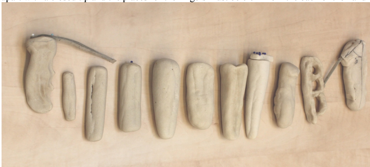
Figure 17. Salt-dough models, where the outer two handles have cardboard extrusions.
