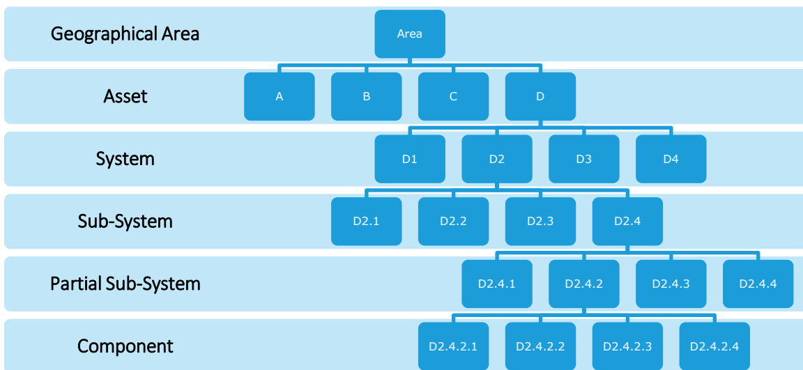
Figure A6.2: Conceptual design of the decision-support method: step 2
