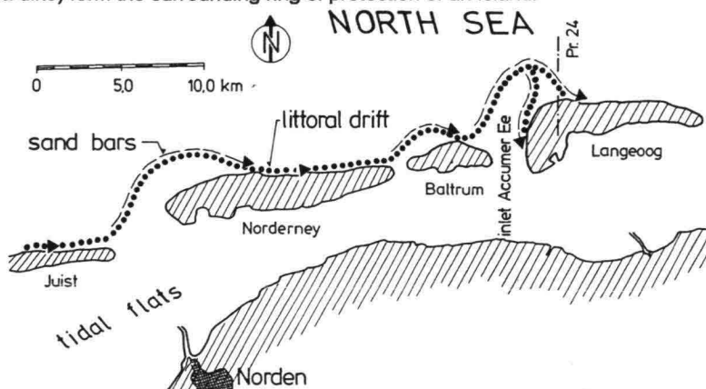
fig. 4: Longshore transport along the East Frisian islands with a reef arch in front of the single strait [4].
