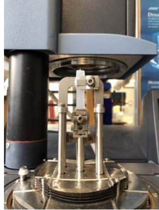
(b) Plate clamped in a tensile machine
