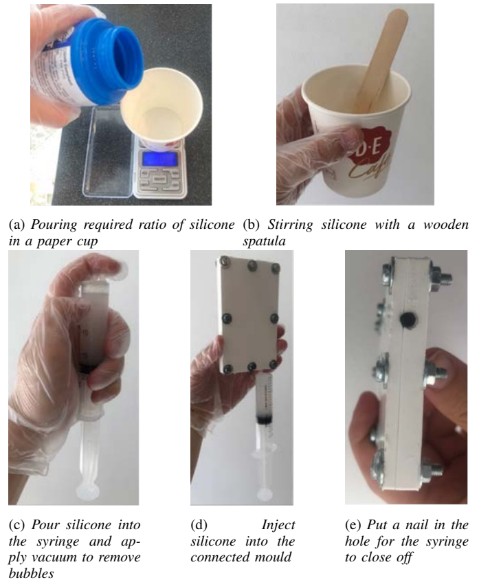
Figure 27: Producing silicone plates by use of the 3D printed mould.
