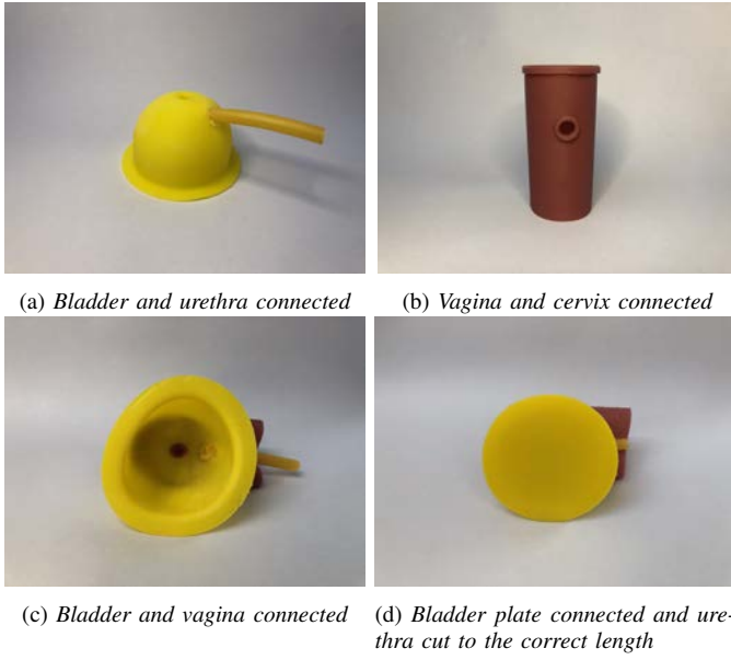
Figure 5: Intermediate stages in connecting the silicone parts.
