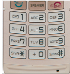
Figure 4.1: The telephone pad showing informal mapping between the set of digits and the set of characters
