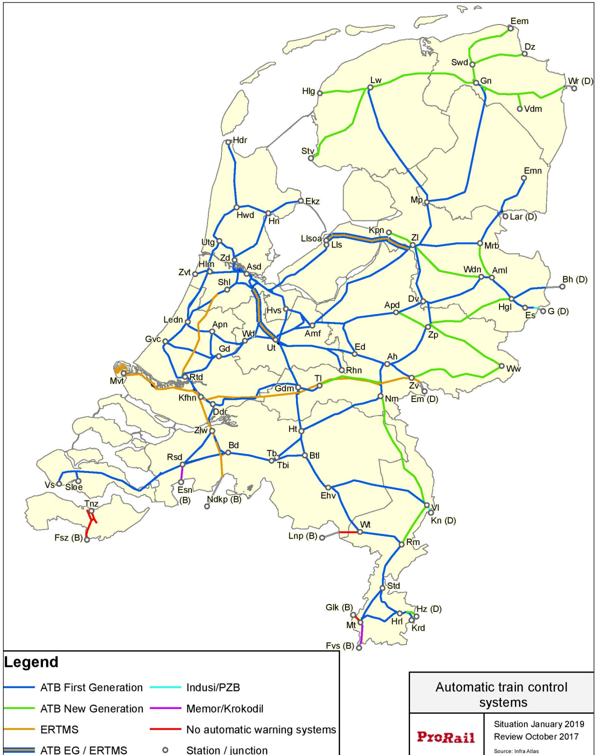
Figure C.7: Automatic Train Control Systems (Prorail, 2018)
