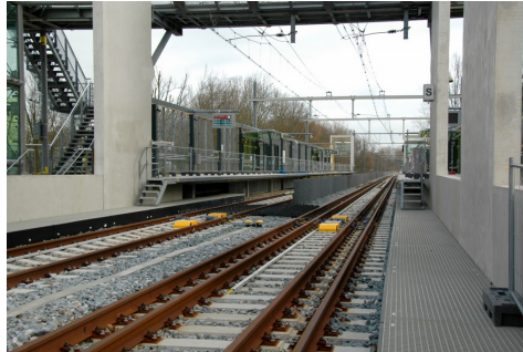
Figure 4.2: The Gauntlet Track at Schiedam Station (Gemeente Rotterdam, 2018)
