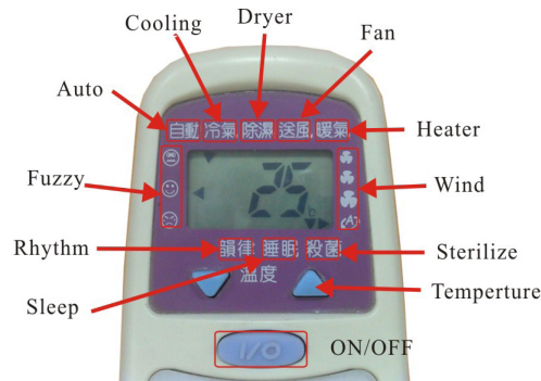
Figure 2 AC controller key functions.
