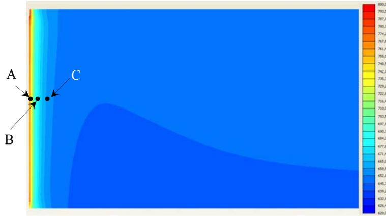
Fig. 6.4: Visualisation of void ratio distribution after jacking phases (phase 6) for HP
