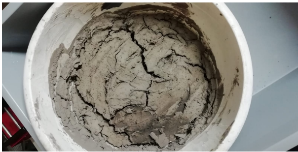
Figure B.4: The clay sample after 110 hours ( \approx 4.5 days) of drying outside.
