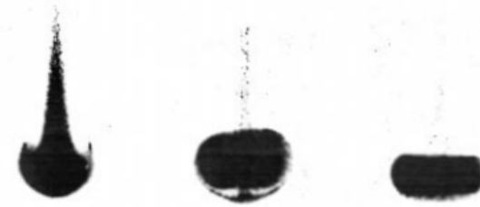
Figure 1.1: Different stages of drop evolution, swarm consists of glass particles in glycerin. Taken from (Machu et al., 2001).
