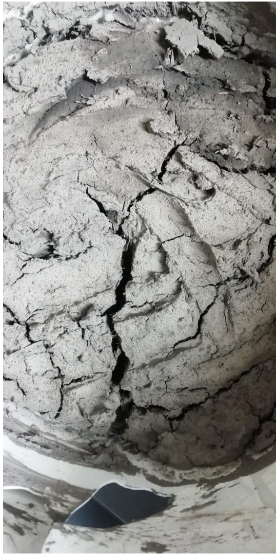
Figure B.6: The clay sample after 110 hours, detailed image of the largest fracture.
