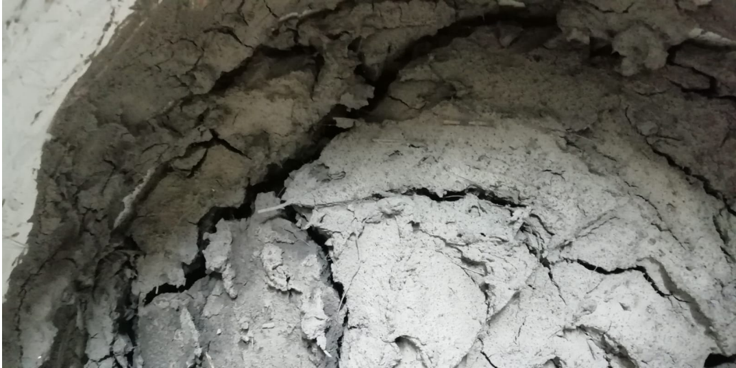
Figure B.8: The clay sample after 110 hours, detailed image of some smaller fractures at the side of the sample.
