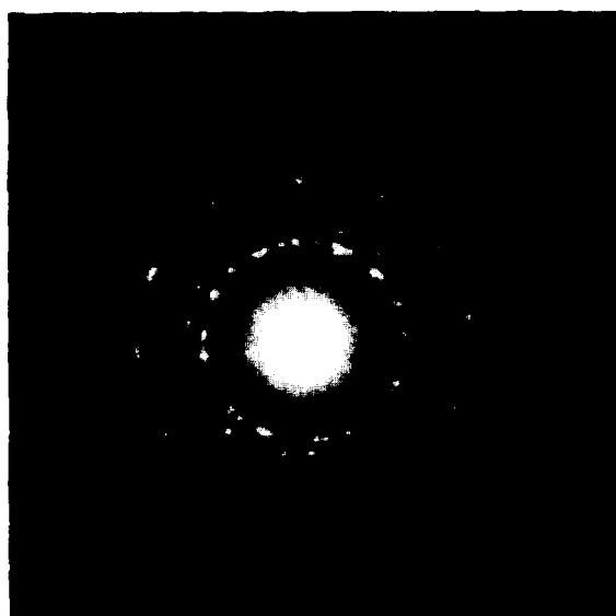
Fig. 8. Electron diffraction pattern for a thin film of \text{LiMn}_2\text{O}_4 .
