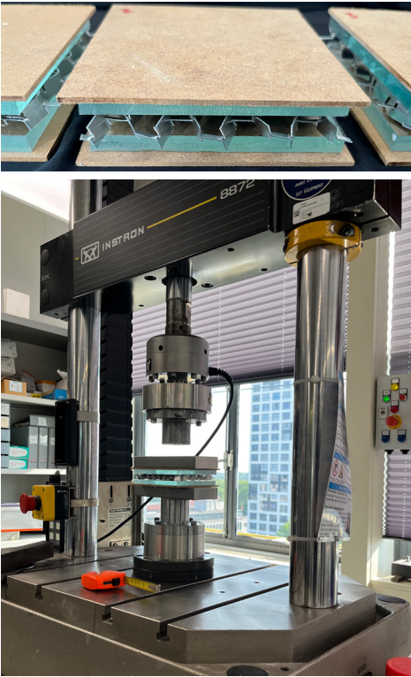
Figure 105: (above) samples; (below) Compression test set-up
