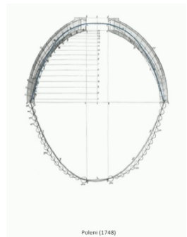
Figure 22: Use of Tension-compression analogy and graphic statics to solve equilibrium. Right: models from Gaudi, Heinz Isler *
