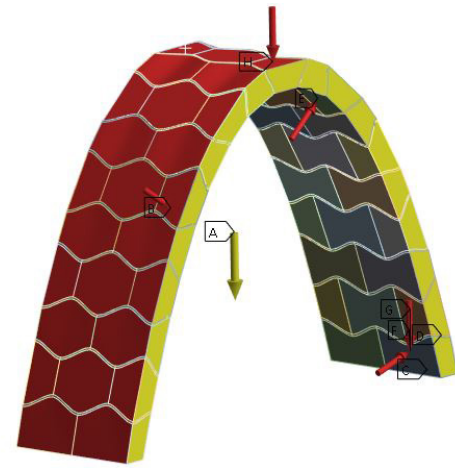
Figure 92: Boundary conditions for Vault under eccentric load
