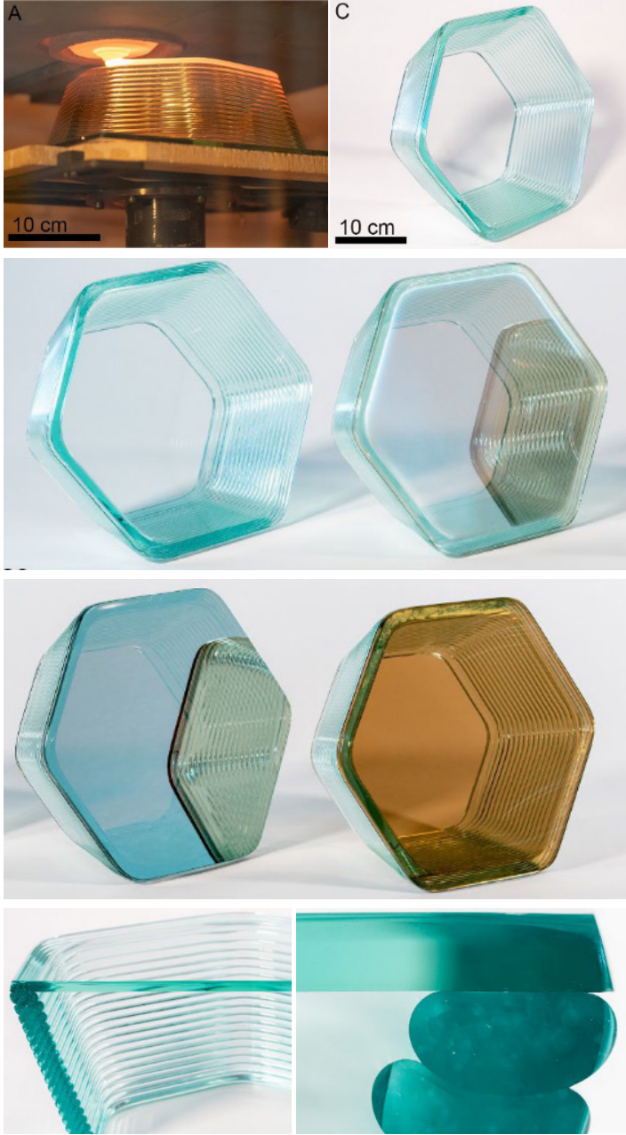
Figure 20: Hexagon form printed on Optifloat float glass and high temperature coated float glass (Source: Stern et al., 2024)
