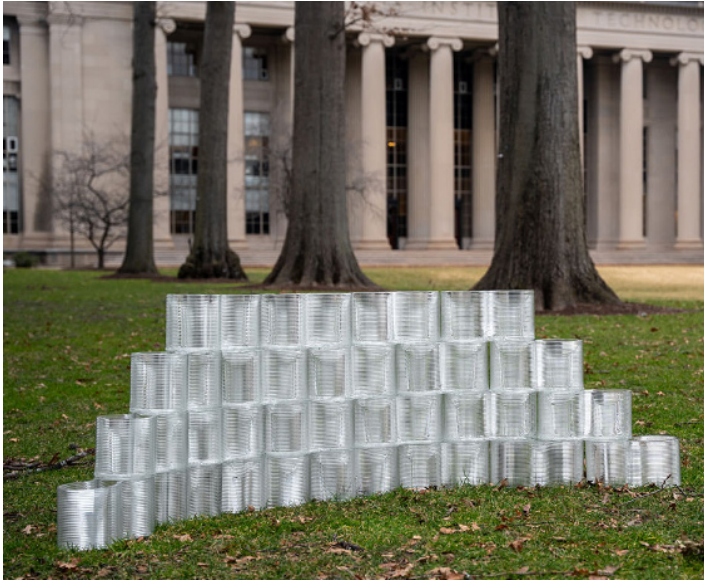
Figure 19: Interlocking units assembled in a Wall configuration (Source: Massimino et al., 2024)
