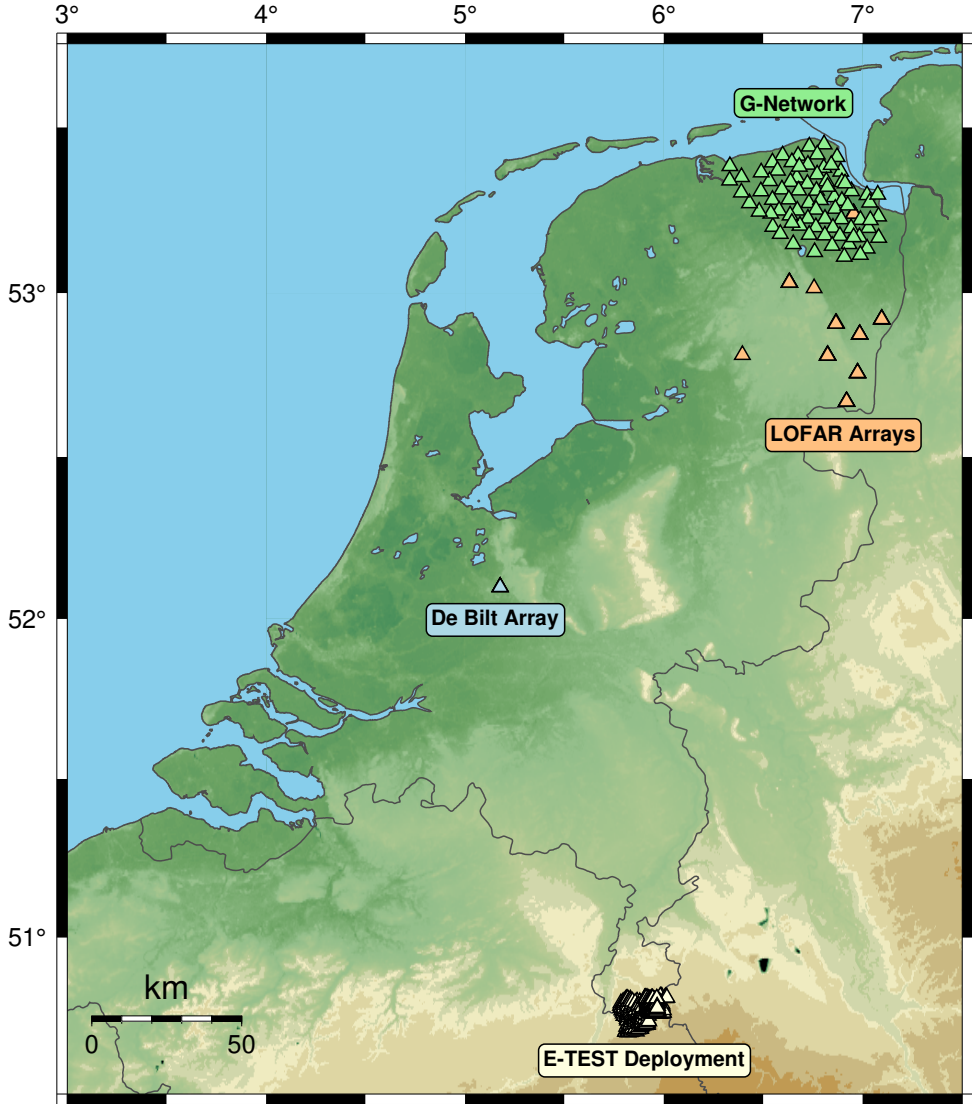
Figure 3.3: Map of the Netherlands showing four groups and locations of geophysical instruments in the field (G-Network – geophones and surface accelerometers; E-TEST Deployment – battery operated geophone nodes; LOFAR – seismo-acoustic array; De Bilt – acoustic array). Further details on the instruments are provided in table 3.1
