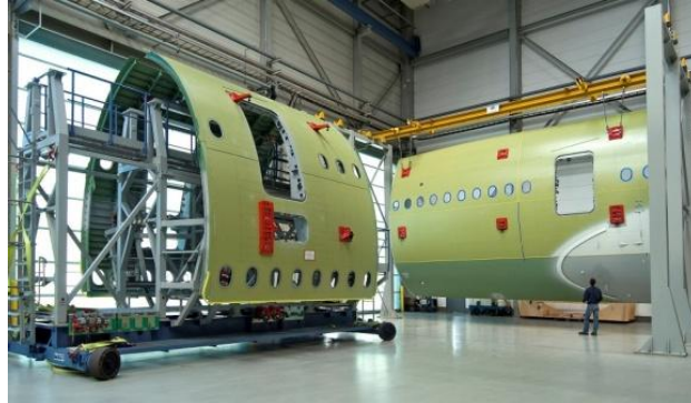
Figure 1.4. Partial GLARE in fuselage of Airbus A380 [17].
