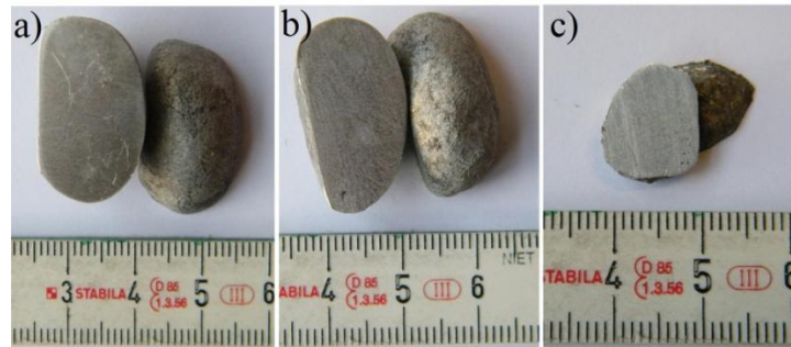
Figure 3.27. 2024 Al alloy inner morphology after refining with flux 44%NaCl-56%KCl-10%Na 3 AlF 6 , and the weight ratio of NaCl-KCl salts mixture to 2024 Al scrap is 1.5:1, 1:1 and 0.5:1, respectively.
