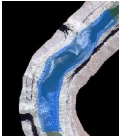
(Left) Modelled area includes a sandbar in the centre, two constrictions and a pool around the sandbar. (Right) Curvilinear grid, 100 by 30 cells, each 12 by 4 m
